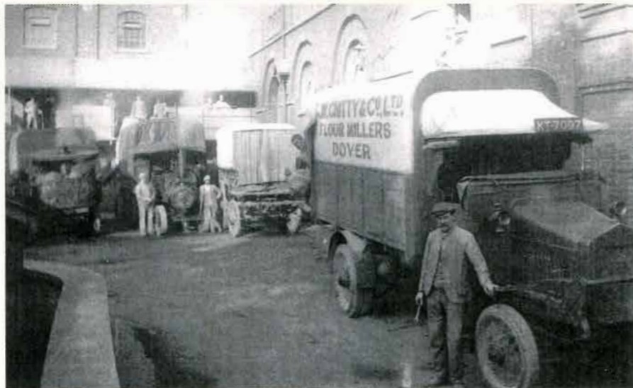
Above: G W Chitty, flour millers of Charlton by Dover, operated this 1915, Hallford seen at the mill in company of a Standard Sentinel and early Foden. The original Hallfords were derived from the Saurer.
